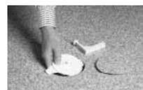
4. Remove the foot of the Phlexiknife in the gully.
