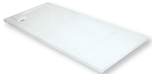
The 1800mm Quick Fit Shower tray can be cut down to a minimum of 1500mm as there are metal strengthening bars that cross the tray at 100mm intervals and comes complete with end panel section. This allows greater flexibility for onsite conditions and allows one tray to be provided for many different scenarios, e.g a 1560mm alcove can be catered for by cutting an 1800mm tray to the exact size required and then fixing the finished end panel section. .
