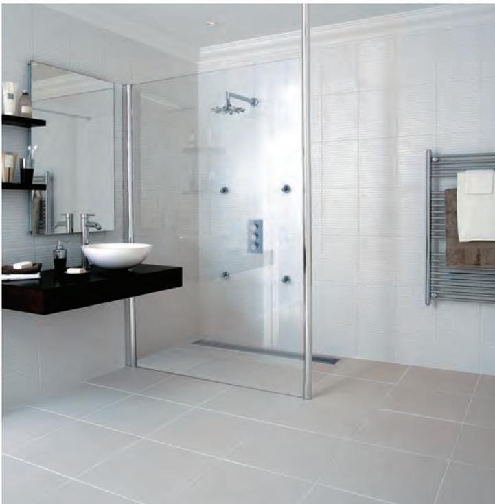
Premier Shower Deck is the perfect solution for use in wet rooms. With built in falls, the gradients in the deck encourage the swift removal of waste water.
