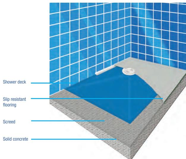
The Premier Shower Deck can be installed into an existing concrete floor by removing the screed and setting the floor former in a position to leave it level with the remainder of the shower room floor. When all pipework is complete the whole shower room floor, including the new shower area can be covered with suitable vinyl flooring or tiled.
