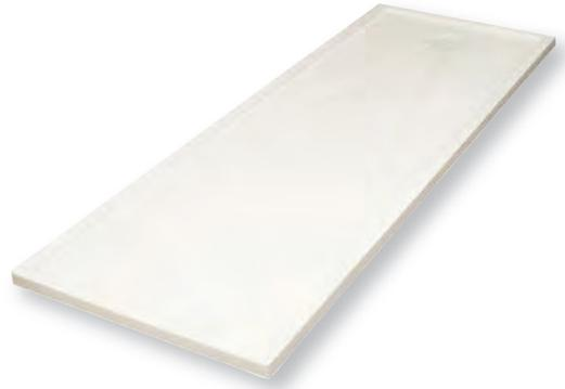
The Universal 1800mm tray can be cut down to a minimum of 1500mm as there are metal strengthening bars that cross the tray at 100mm intervals and comes complete with end panel section.
