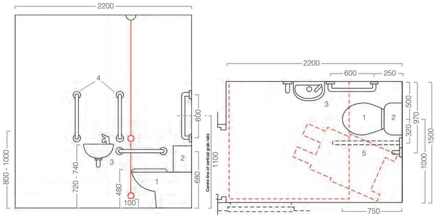
Cistern lever should be installed on the right of the cistern for LH installation and on the left for a RH installation. (Left hand illustrated.)
