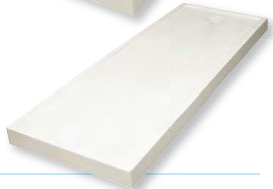
The Easy Fit 1800mm tray can be cut down to a minimum of 1500mm as there are metal strengthening bars that cross the tray at 100mm intervals and comes complete with end panel section.
