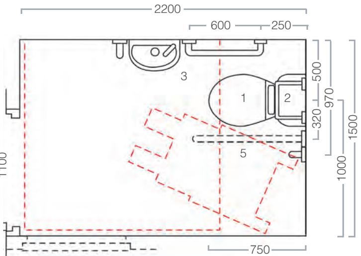
The W.C. pan can be installed as a standard low level configuration with exposed cistern. To achieve this install the W.C. 200mm off the wall. If required the void left could be filled by our laminate spacer box unit see page 170.
