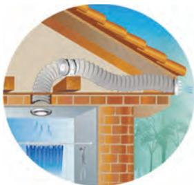
The rate of extraction you require depends on the size of the room and the amount of condensation produced. The bigger the room or if large amounts of condensation are produced, then the more the air will need to be replaced in the room, thus you need a higher rate of extraction.
