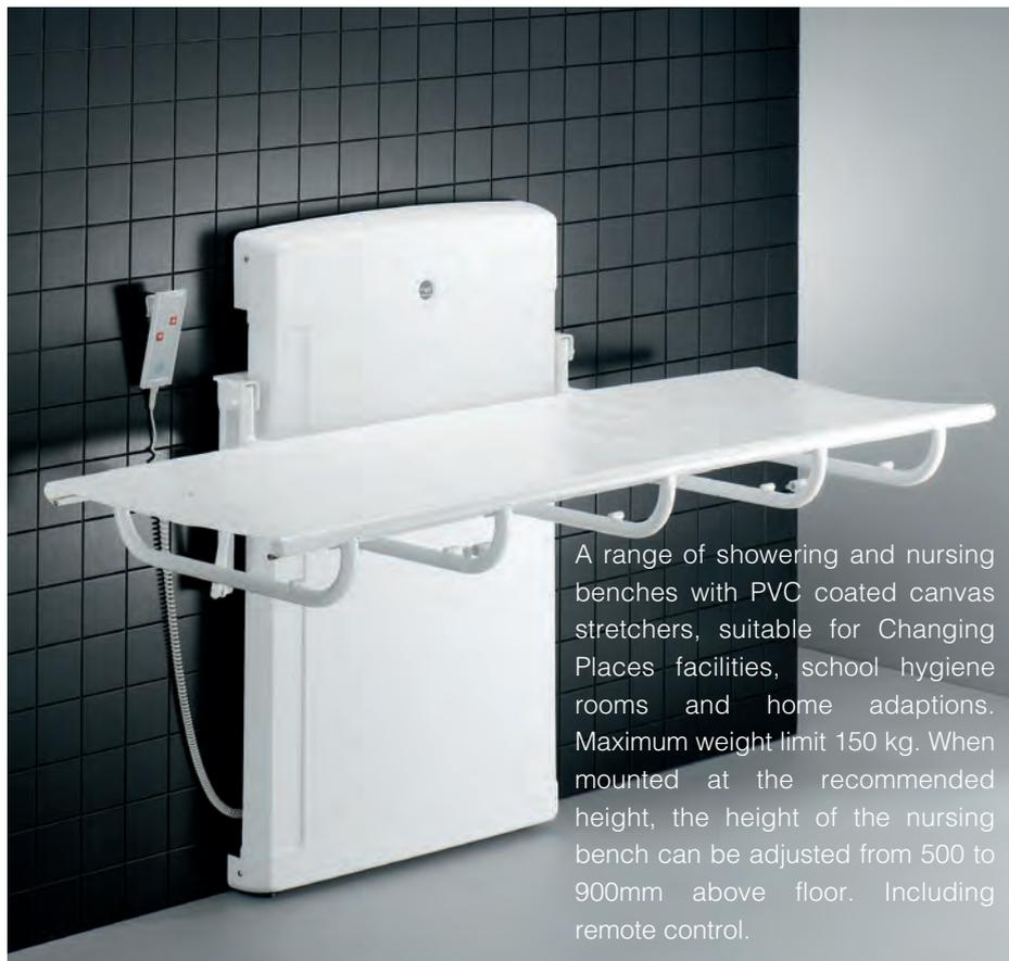
A range of showering and nursing benches with PVC coated canvas stretchers, suitable for Changing Places facilities, school hygiene rooms and home adaptations. Maximum weight limit 150 kg. When mounted at the recommended height, the height of the nursing bench can be adjusted from 500 to 900mm above floor. Including remote control.
