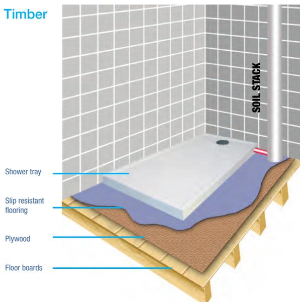
Low level access can be achieved if installing the Easy Fit Shower Tray onto an existing floorboard or chipboard floor, which cannot be breached. The tray can be sited directly onto the timber floor and used in conjunction with a gravity waste with the pipe work concealed beneath the tray.
