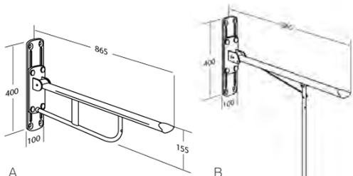
Projection when folded: 200mm. Projection when folded: 155mm.
