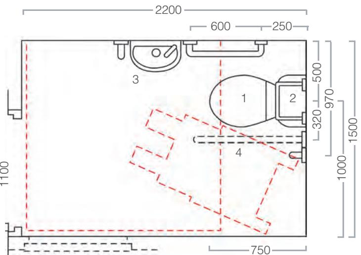
Cistern lever should be installed on the right of the cistern for LH installation and on the left for a RH installation. (Left hand illustrated.)
