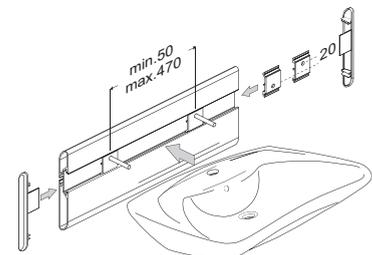
Mounting of wash basin: Bolt-mounted basin. Basin hole spacing: Min. 50mm; max. 470mm. The bolts can be set in positions 1-2 for adjustment of wash basin on the bracket. For bolt mounted wash basin see pages 186 - 190.
