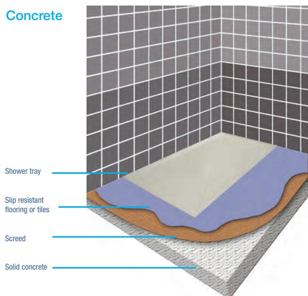
The Floor Line system can be installed into an existing concrete floor by removing the screed. When all pipework is complete the shower room floor area can be covered with a suitable vinyl or tile flooring. The flooring should be butted against the edge of the Floor Line tray and joined with a suitable flexible sealant.
