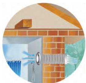
A wall mounted fan is where the fascia has an integrated fan and the ducting passes through the wall to an external grill.
