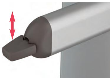
Gas with lever control – lift the lever control to release the lock. Push the basin to required height. Return the lever control to a horizontal position. The wash basin is now locked into the new position.
