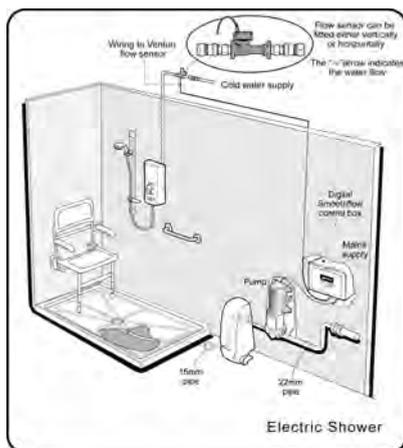
The Digital Smoothflow Kit is designed to minimise gulley suction noise by precisely matching the pump flow rate to the shower flow rate.
