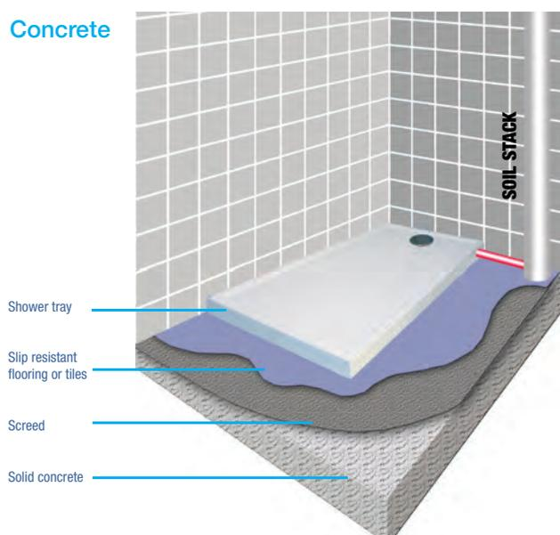
Low level access can be achieved if installing onto existing concrete floors. The Easy Fit Shower Tray can be sited directly onto the concrete or screed subfloor. The unique gravity waste can be installed allowing pipe work to be concealed beneath the tray.
