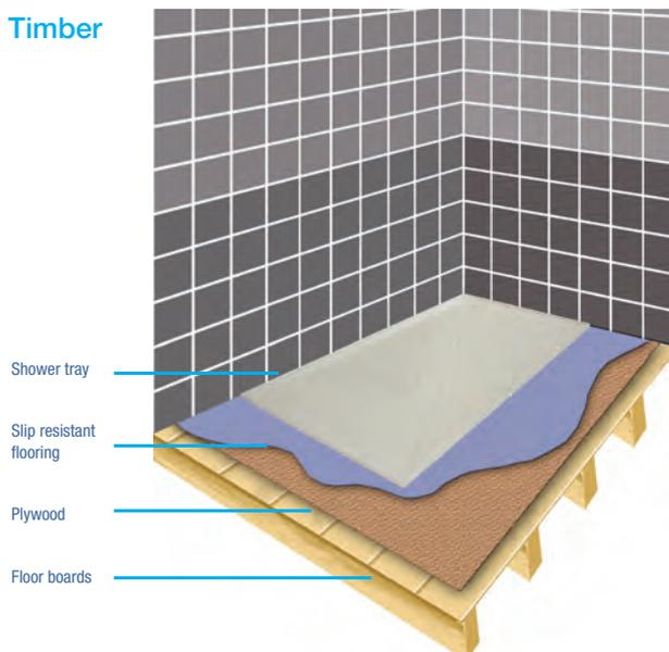
The Floor Line system can be installed into an existing timber floor by removing the floorboards and setting the tray onto the joists and in-fill panels. The tray will then be brought level with the existing floor with plywood to make the whole shower room level.
